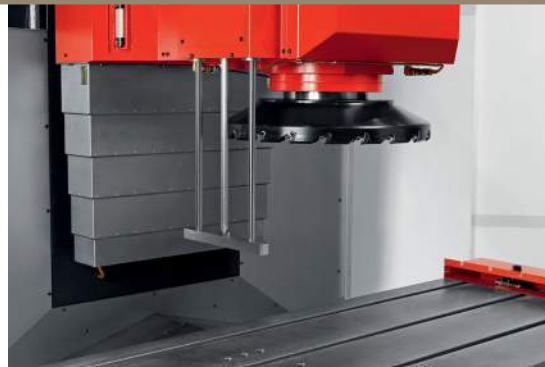
Automatic Measuring System
